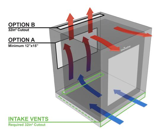
Above is a diagram displaying the (3) cabinet cutout options for a properly ventilated environment. **Both intake vents marked in green are required.**
